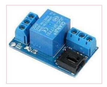
A relay is an electrically operated device. It has a control system and (also called input circuit or input contactor) and controlled system (also called output circuit or output cont actor). It is frequently used in automatic control circuit. To put it simply, it is an automatic switch to controlling a high-current circuit with a low-current signal.
