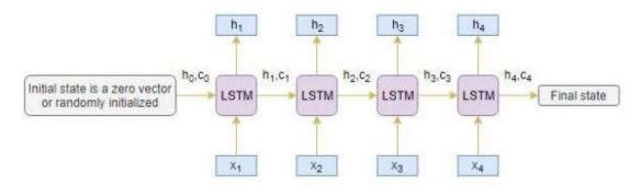
The hidden state (hi) and cell state (ci) of the last time step are used to initialize the decoder.
