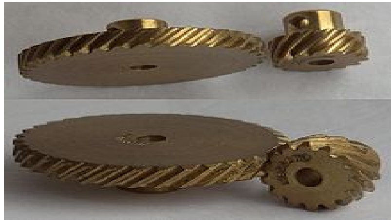
Fig 1.3 - Helical gears, Top - parallel configuration; bottom - Crossed configuration
