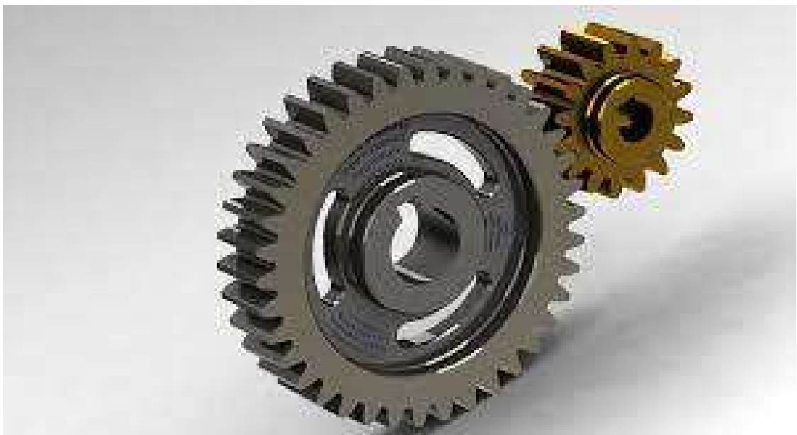
Fig 1.2 - A spur gear and spur pinion in mesh
