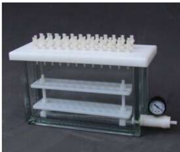
Figure 1.3: Components of solid phase extraction (SPE).
