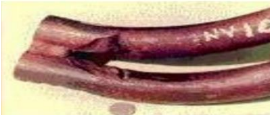
Fig-4 Tube failures because of fatigue failures
