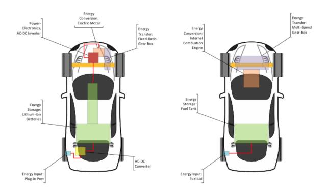
Figure 2- Electric Vehicle vs IC Engine Vehicle
