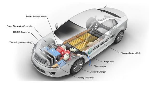
Figure 1- Inside an Electric Vehicle
