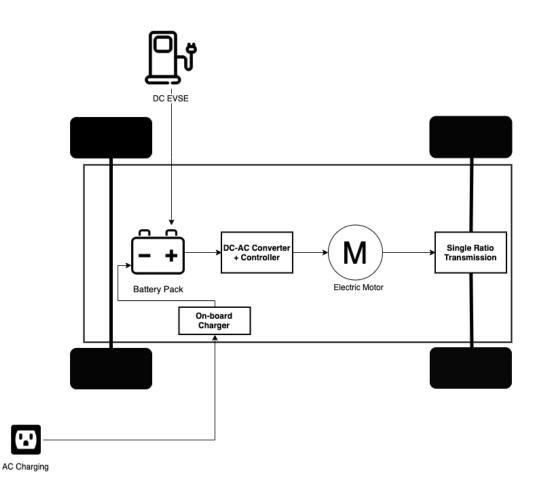
Figure 3- Components of an Electric Vehicle
