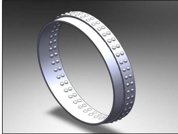
Fig 4. 3D CAD model of boiler shell joint
