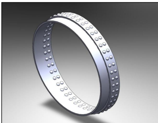
Fig 1. 3D CAD model of boiler shell joint
