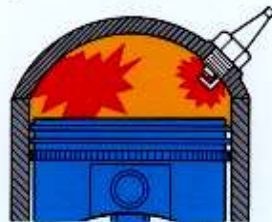
Spark plug "fires" and two flame fronts form.
