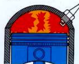
Spark knock occurs because of excessive pressure in cylinder.
