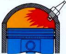
Normal combustion spreads very slowly.
