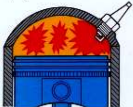
Flames collide with pressure "spike" and knock.
