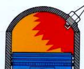
Piston moves toward flame front.
