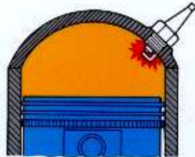
Spark occurs, combustion is slow but normal.
