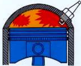
Both flame fronts shoot toward each other at high speed.
