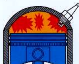
Two flames collide, causing pressure "spike" and knock.
