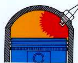
Pressure builds as piston slams into combustion flame.
