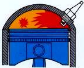
End gas auto-ignites and two flame fronts spread rapidly.
