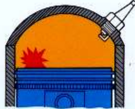
Hot carbon deposit ignites fuel mixture.
