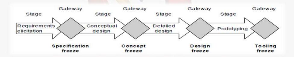
A design freeze is a binding decision that defines the whole product, its parts or parameters and allows the continuation of the design based on that decision.
