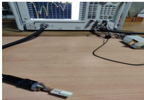
Fig. 4.10: Experimental test set up of the measurement of Return loss, VSWR, Z_{in} , and Smith chart
