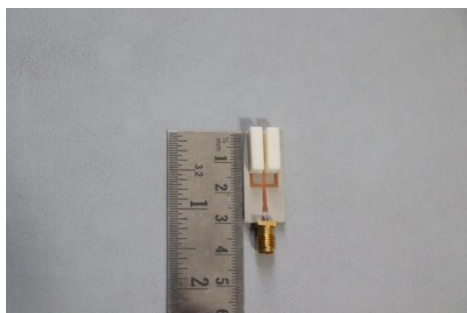
Fig.3.2: Top 2-D view of the proposed Rectangular DRA
