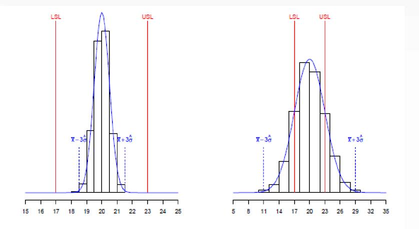
The two distributions have same mean and specification limits. However, dispersion in the distribution on the right is higher. Therefore, the process capability of the distribution on the right is lower than the process capability of the distribution on the left.
