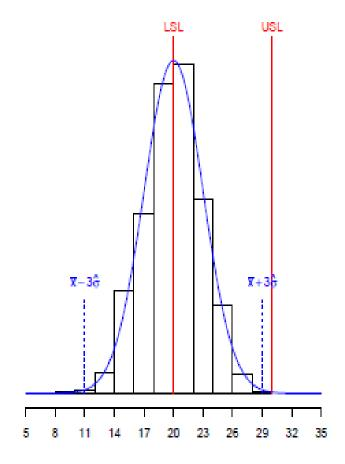
The two distributions have the same characteristics as far as shape, position and dispersion are concerned. The limit spread is the same. The process on the right is not centered with respect to its specification limits. Therefore process capability on the right will be lower.
