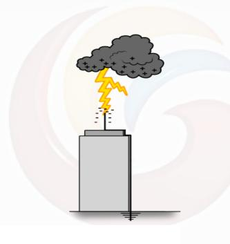
Lighting Rods are connected to the ground. When a cloud carrying electric charges approaches, the rod attracts opposite charges from the ground. The Electric field at the tip of the rod is much stronger than anywhere else. When the E-field exceeds the air breakdown strength (of 33 kV/cm), charges start to travel to ground.
