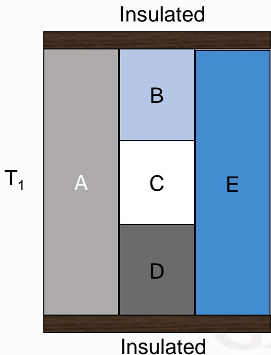
$$Q = \frac{T_1 - T_2}{R} \quad W$$
