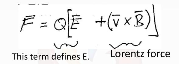
There are electromagnetic forces that depend on the velocity of a charge in given fields, and these forces are perpendicular to **v**. This term defines a field "B", which is the macroscopic magnetic field, or "Magnetic Induction".
