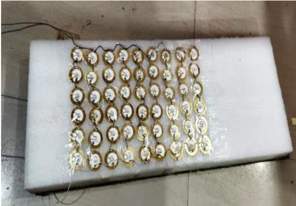
Fig.14: Piezo-plates matrix setup over a hard foam surface
