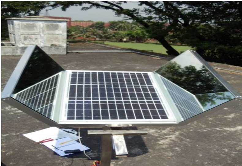
Fig.6: Solar Panel with two-side mirror
