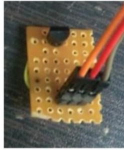
Fig 4.5.(c). Body temperature sensor
