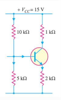
$$V_{CE} = V_{CC} - I_C (R_C + R_E)$$
