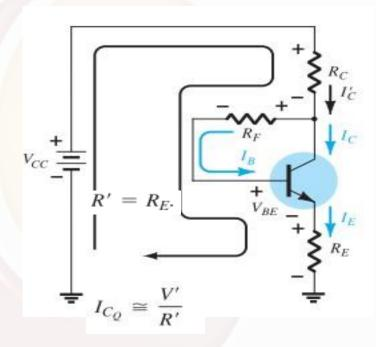
$$I_B = \frac{V_{CC} - V_{BE}}{R_F + \beta (R_C + R_E)}$$
