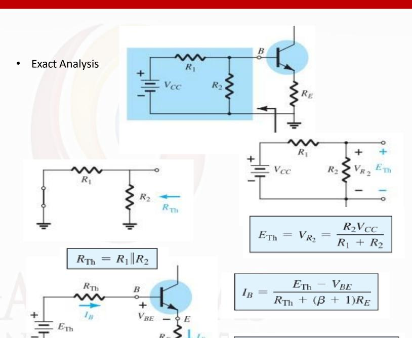
$V_{CE} = V_{CC} - I_C(R_C + R_E)$
