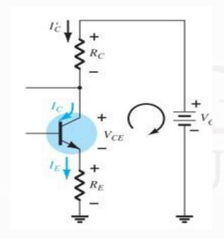
$$I_E R_E + V_{CE} + I_C' R_C - V_{CC} = 0$$
