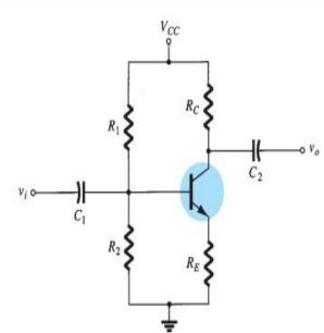
• DC components of the voltage-divider configuration.
