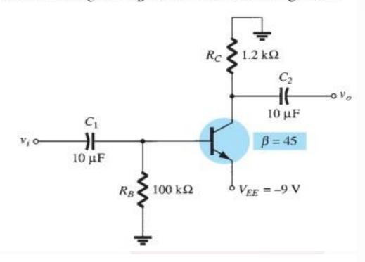
**Solution:** Applying Kirchhoff's voltage law in the clockwise direction for the base–emitter loop results in
