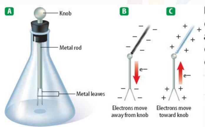
Notice the position of the leaves on the electroscope when they are (1) uncharged, (1) negatively charged, and (3) positively charged.
