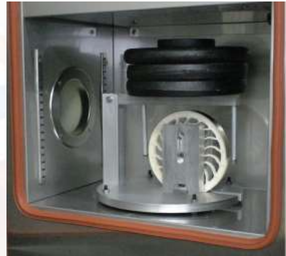
Wheel prototype under load during creep testing
