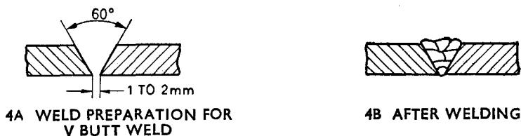
FIG. 4 SINGLE-V BUTT WELD WITHOUT REINFORCEMENT
