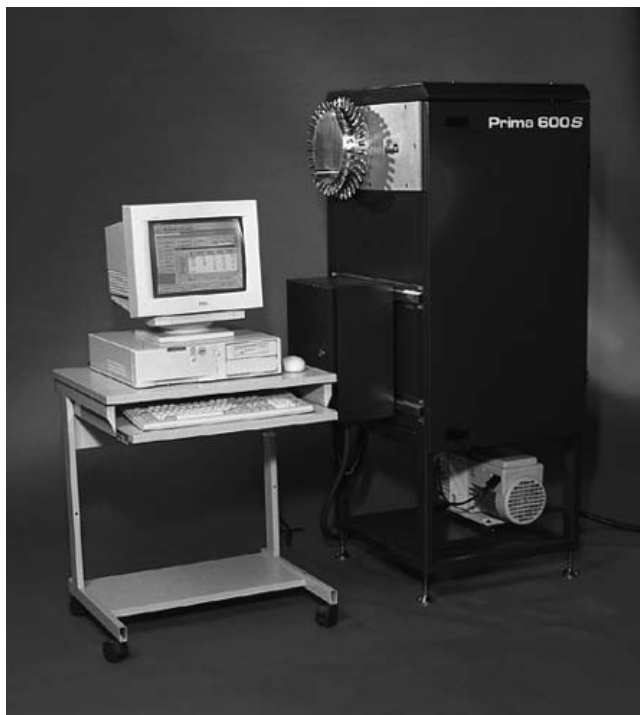
Figure 7. Magnetic sector mass spectrometer unit from VG Gas Analysis Systems Ltd. fitted with the rotary motor sample device.
