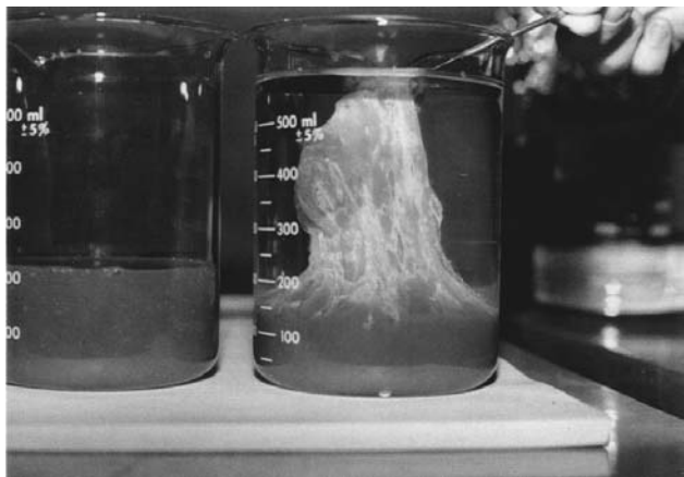
Figure 3. Solvent precipitation of pullulan: Pullulan, which is soluble in the fermentation broth (yellow solution), becomes insoluble in methanol (clear liquid). The fibrous texture appearance of the precipitated pullulan indicates that this polysaccharide has very high molecular weight.
