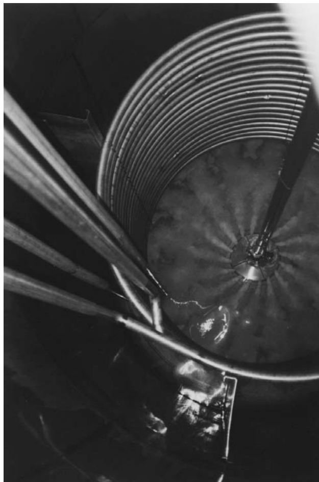
Figure 2. How the Frings Aeration System works. Acetator filled for demonstration with a small amount of water immediately after the start of the aeration. Air is aspirated through the suction pipe from the top and the formed emulsion is spread out in beams at the bottom of the fermenter, reaching the wall of the fermenter somewhat outside of the cooling coil.
