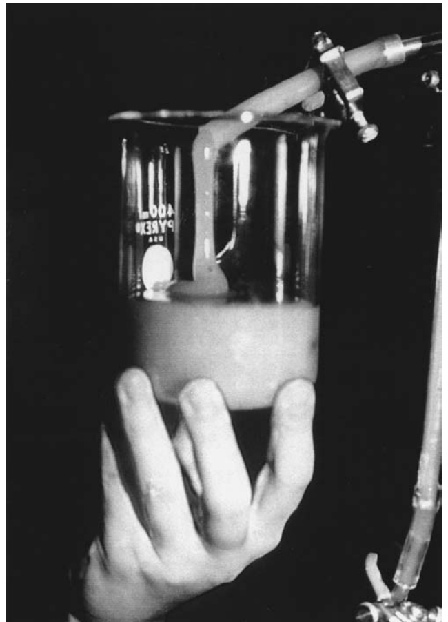
Figure 8. Highly viscous fermentation broth of A. pullulans in a sucrose medium: the broth slowly flowing out of a fully opened large-size sampling tube under the compressed air inside the fermenter.
