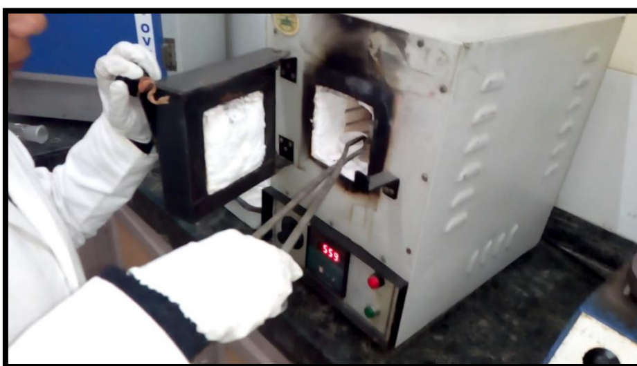
Fig. 2 Testing procedure for acid insoluble ash
