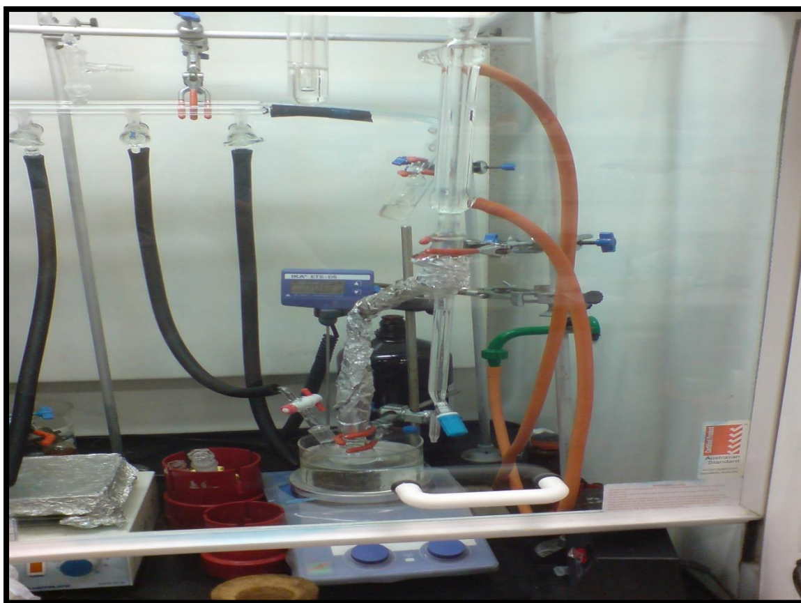
Fig. 1 Dean and stark distillation apparatus
