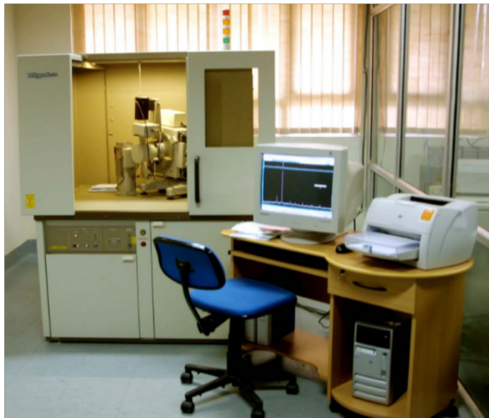
Fig. 3.1: Powder XRD system (Make: Rigaku; Model: DMax 2200)
