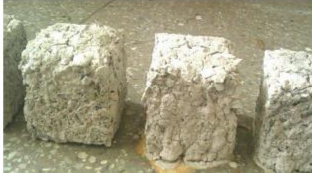
Figure 4. 8 Fractured Cube Specimen after 28 days in H 2 SO 4
