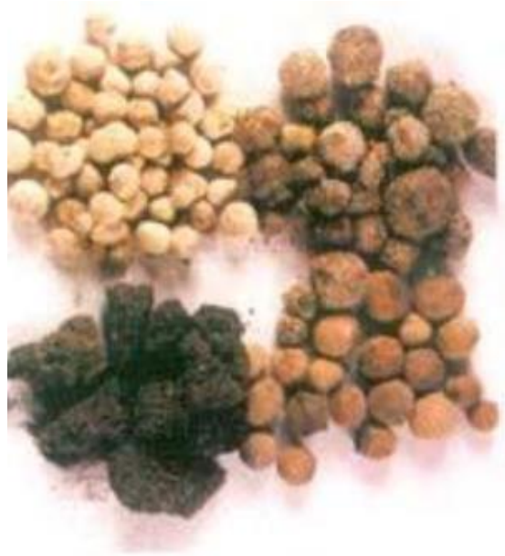
Figure 1.3 Pelletized and sintered fly ash makes a good lightweight aggregate
