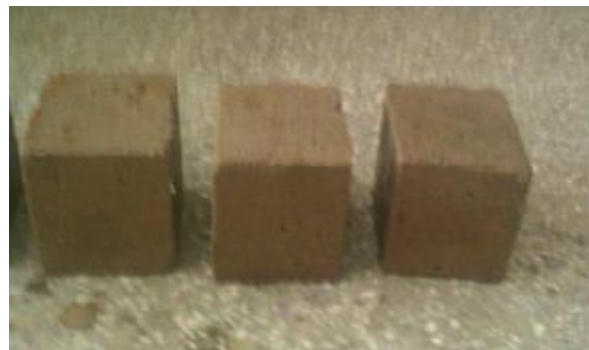
Figure 4. 7 Cube Specimens after 28 days in HNO 3
