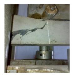
Fig.1 Diagonally placed tesile failure
