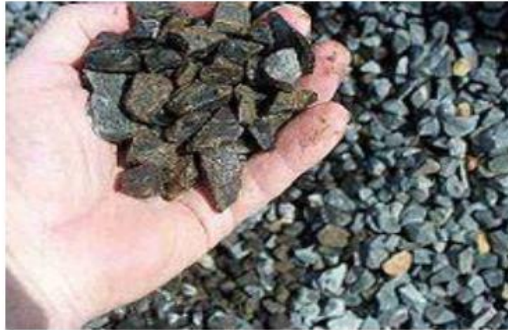
Figure 4. 2 Recycled concrete aggregates after processing
