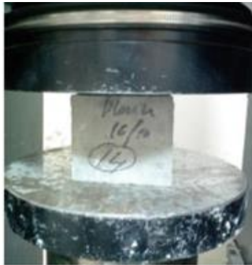
Figure 4. 7 Experimental setup for compressive strength; (a) Cubical test
