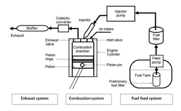
Figure 2.2.1 : Schematic diagram of a typical diesel engine fuel system
