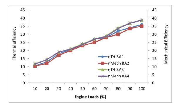
Figure 2.2.2 : Effects of engine loads on thermal and mechanical efficiencies
