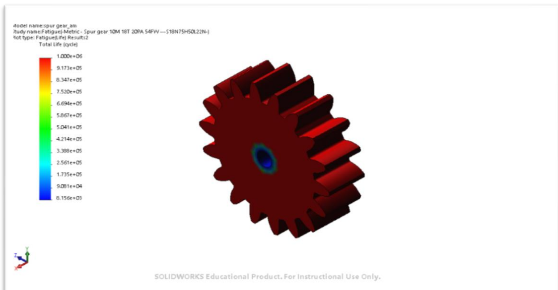
Fig. 8 fatigue result of polycarbonate
