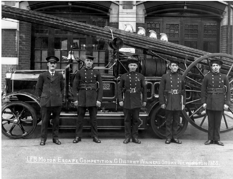
Figure 6.6 London Fire Brigade wheeled escape ladder and crew. The caption reads: London Fire Brigade motor escape competition G. District winners, Stoke Newington, 1925. © Mary Evans Picture Library.
