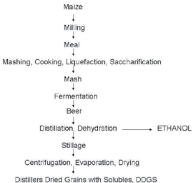
Fig 4.5 Ethanol production from maize (dry-grind process)
