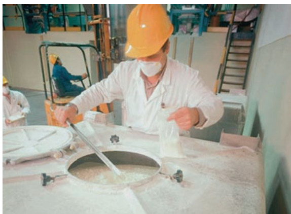
Fig. 2 Slurry in the stainless-steel holding tank of the Microfluidizer after continuous high shear fluid processing of chitosan powder for mechanical disassembly into nanofibrils. Scaleable results are produced for pilot and production purposes
