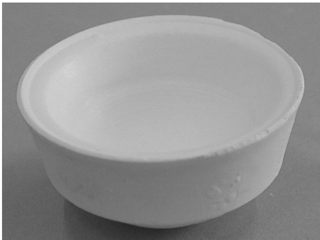
Figure 10.16. FGM cup insert, made by EPD. [Anné, 2005a].
