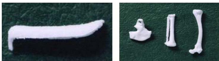
Fig. C.3 Photographs of nasal prosthesis and bone-shaped polymer scaffolds prepared by bone-shaped silicon moulds.
