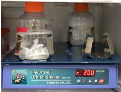
Fig. L.1 Tissues immersed in the decellularising solution with continuous shaking at 200 rpm using an orbital shaker.
