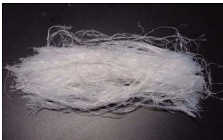
Fig. O.6 Dry chitosan fibres.
