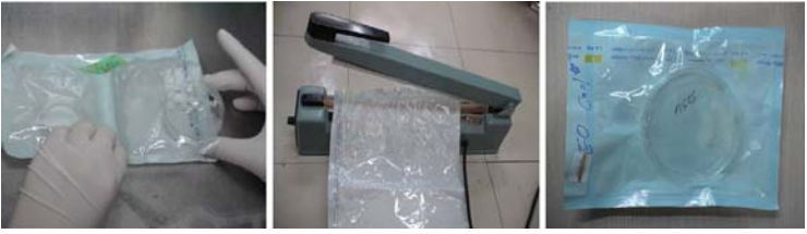
Fig. V.1 Package procedure of scaffold.
