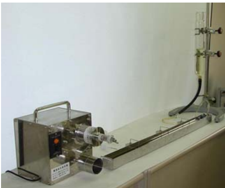
Fig. O.3 Photograph of multifilament spinning system.
