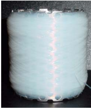
Fig. O.5 Wet spun chitosan fibre bundle.
