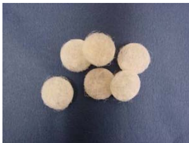
Fig. O.8 Photograph of chitosan fibrous matrix.
