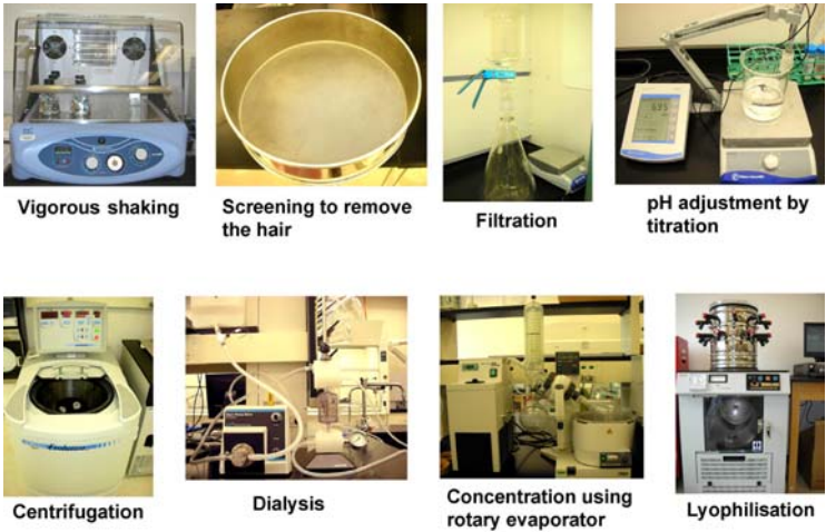
Fig. M.1 Equipment used for keratin biomaterials processing.
