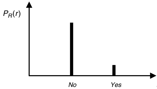
Figure 10.1. Histogram showing probabilities of the values of the discrete random rainfall event variable R .
