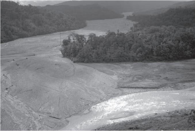
Figure 27.2. Photograph of the junction of the Ok Mani (left) and Ok Tedi (right). The Ok Mani receives the waste rock pushed into the Harvey Creek valley. The large volume of sediment, completely burying the original valley floor, has altered the morphology of both rivers. (Photo by Ian Campbell.)
