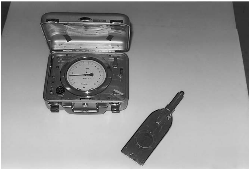
FIGURE 28.3 A dilatometer. (Picture courtesy of A. Bernal and A. Karim, Bechtel Geotechnical Laboratory, Purdue University.)
