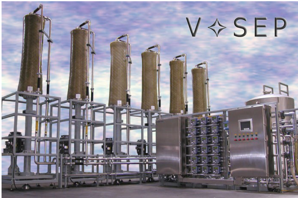
Fig 23. Industrial VSEP modules with 150 m² of membranes
