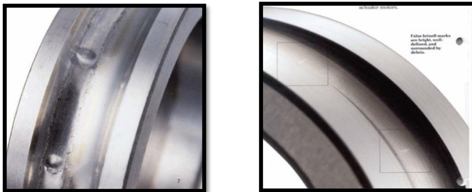
Figure 12: defects due to brinelling [17]
