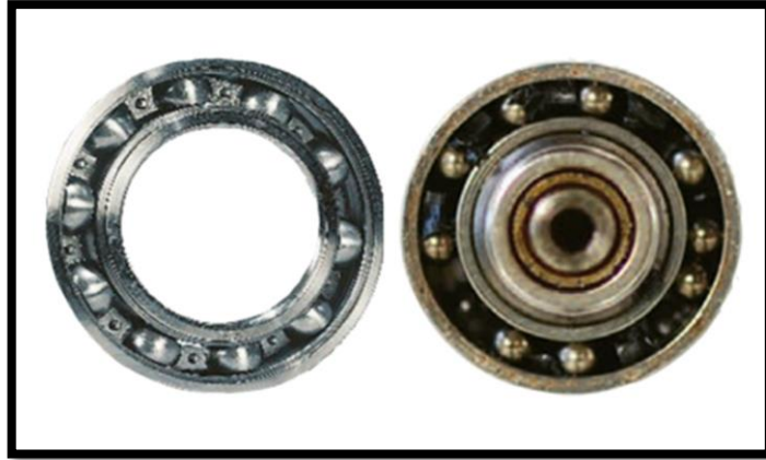
Figure 3: Healthy and defective Ball Bearing
