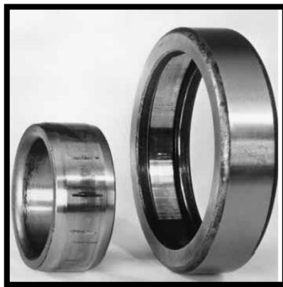
Figure 10: Roller bearing defect due to corrosion [17]
