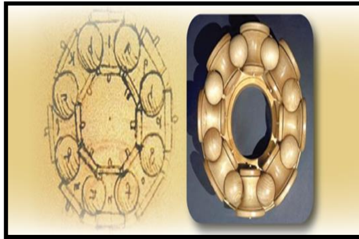
Figure 2: Ball bearing design invented by Leonardo da Vinci [4]
