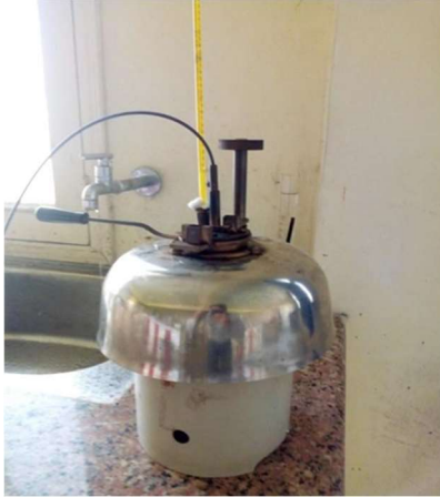
Fig: Pensky-Marten Apparatus to determine the Flash and Fire Point of a sample.
