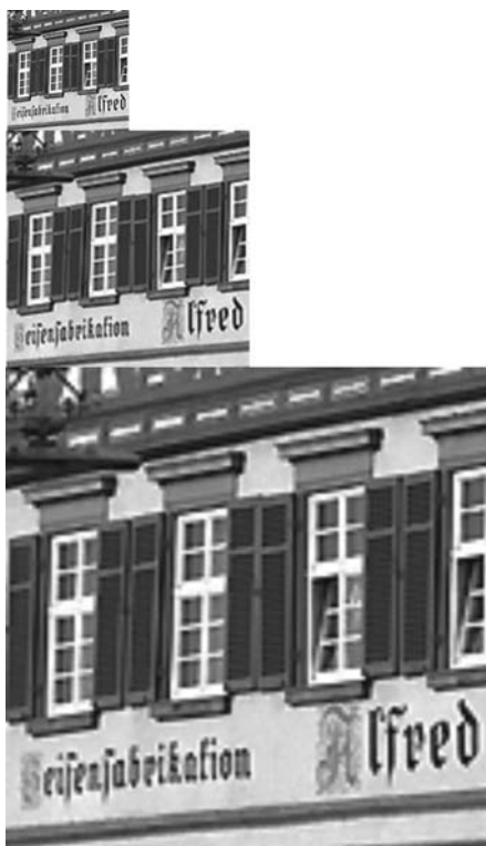
Fig. 15.10. Zooming in by factors of two and four, using the Bartlett filter.
