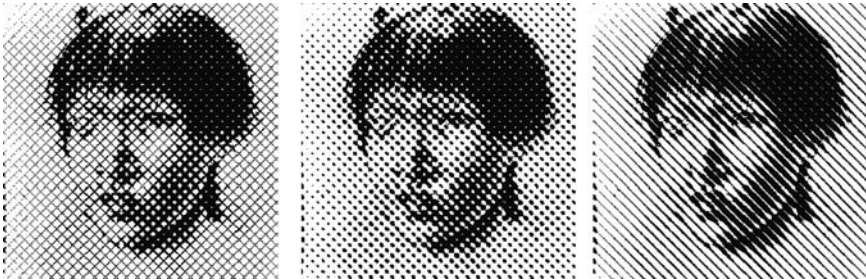
Fig. 12.15. Changes in the dithering matrix lead to different geometries for the pixel clusters.
