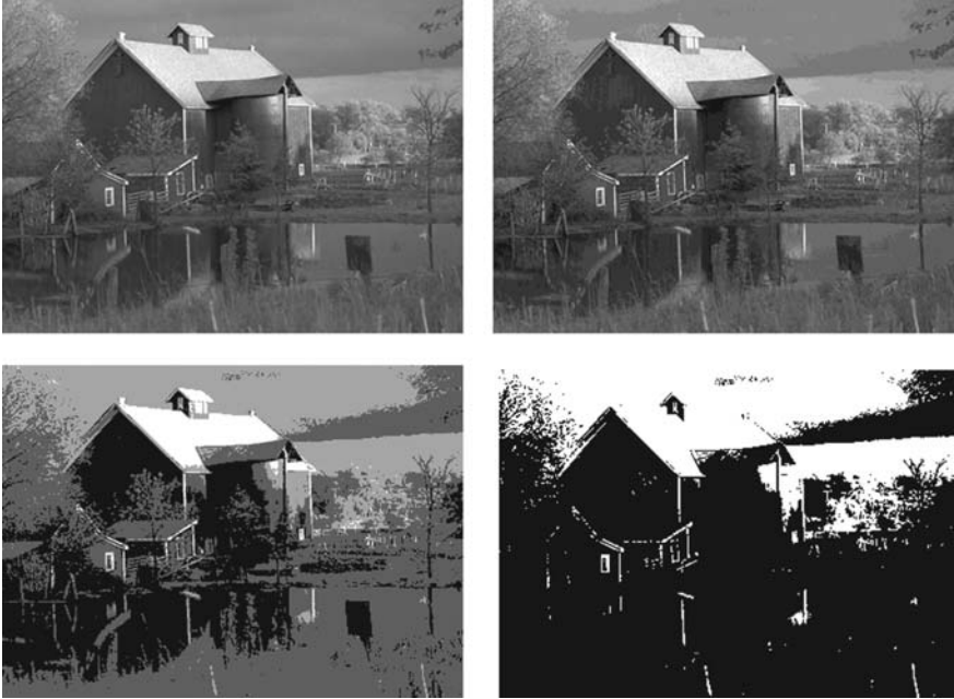
Fig. 11.4. Quantization contours under different numbers of quantization levels: (a) 256; (b) 16; (c) 8; (d) 2.
