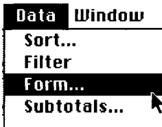
Figure 1.116 Menu items Data and Form... to convert a worksheet into a database form.
