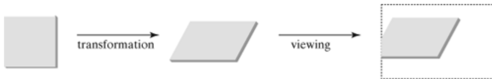
Figure 2.1. A 2D graphics object is processed in a pipeline of transformation and viewing.
