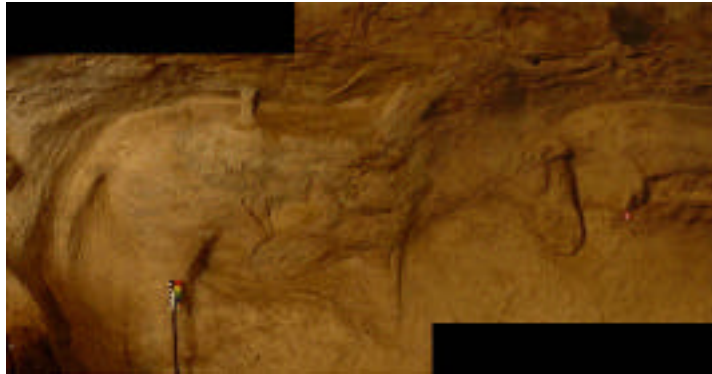
Figure 7.16: Photograph of cave site with photogrammetric reference card and laser scan point
