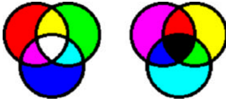
Figure 5.6: emissive colors (left) and transmissive colors (right)
