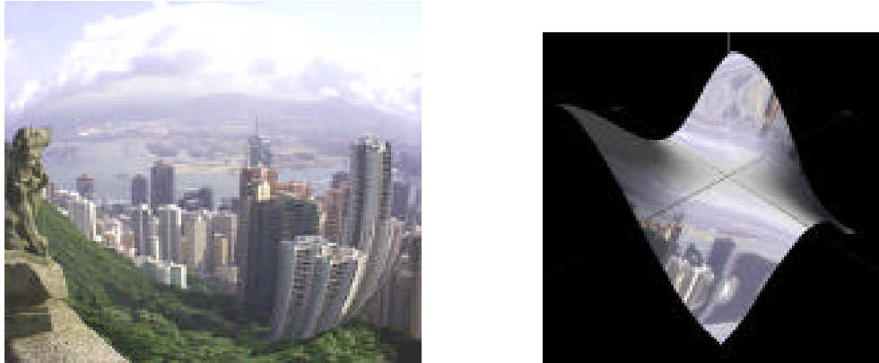
Figure 11.13: the original texture for an environment map (left) and the map on a surface (right)
