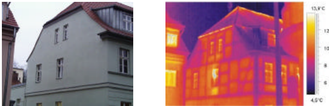
Figure 6.4: A house shown in a normal photograph (left) and with thermal imaging (right)
