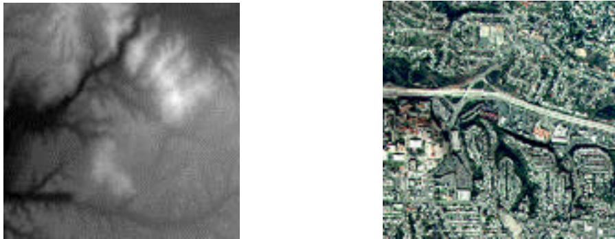
Figure 7.14: height field from USGS digital elevation map (left) and texture map of a portion of the same space from aerial photographs, courtesy of Jeff Sale, San Diego State University
