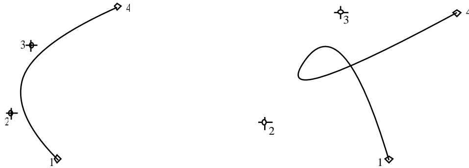
Figure 15.10: two spline curves that illustrate the shape of the curve with different layouts of control points
