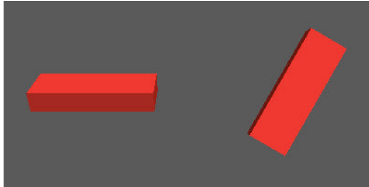
Figure 2.7: the results from two different orderings of the same rotations
