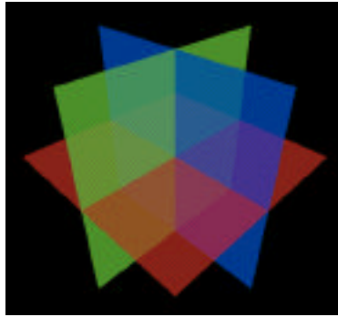
Figure 5.13: the partially transparent planes broken into quadrants and drawn back-to-front
