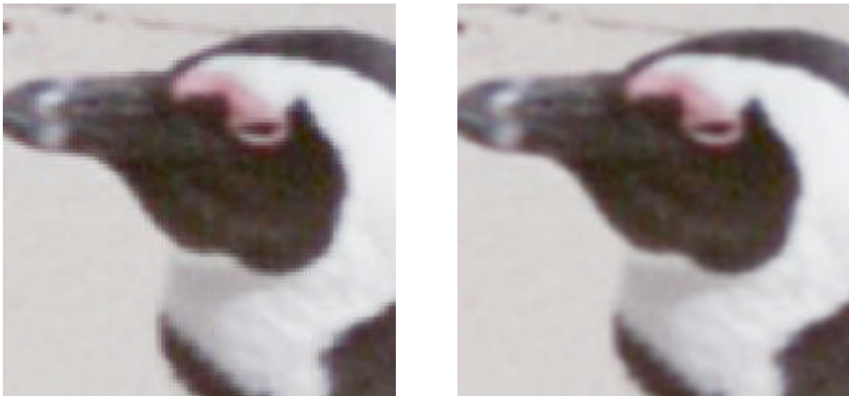
Figure 11.10: the penguin head texture with the GL_NEAREST (left) and GL_LINEAR (right) magnification filters
