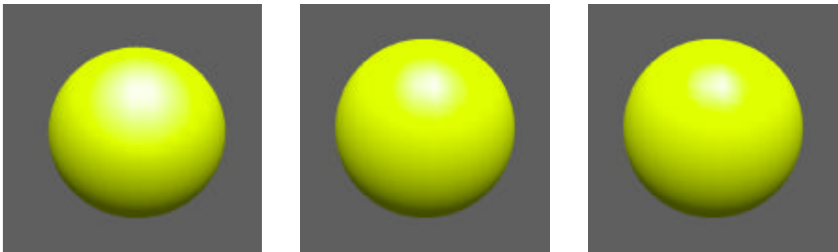
Figure 9.3: specular highlights with specular coefficients 20, 50, and 80 (left, center, and right), respectively
