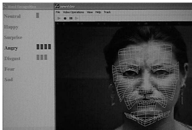
Figure 7.2. A snap shot of the realtime facial expression recognition system. On the right side is a wireframe model overlayed on a face being tracked. On the left side the correct expression, Angry, is detected (the bars show the relative probability of Angry compared to the other expressions). The example is from Cohn-Kanade database [Kanade et al., 2000].
