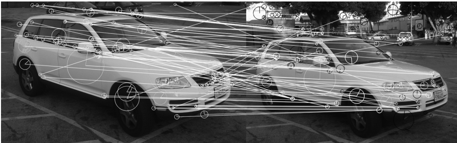
Figure 16-36. Here SIFT keypoints and their descriptors are extracted for two views of the same automobile. Matches were generated using a FLANN-based matcher and visualized with cv::drawMatches() . Matches that were found are marked in white with a line connecting the corresponding features. Keypoints in either image that were not found to have a match are indicated in black
