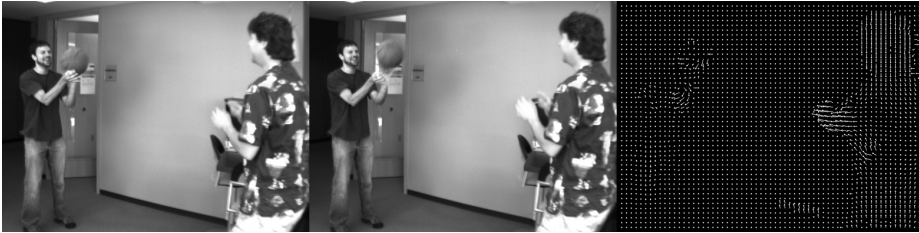
Figure 17-2. Motion from the left and center frames are compared, and represented with a field of vectors on the right. The original images were 640x480, winsize=13, numIters=10, polyN=5, polySigma=1.1, and a box kernel was used for pre-smoothing. Motion vectors are shown only on a lower density subgrid, but the actual results are valid for every pixel
