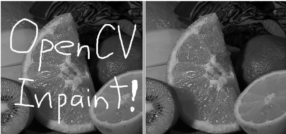
Figure 11-8. An image damaged by overwritten text (left) is restored by inpainting (right)
