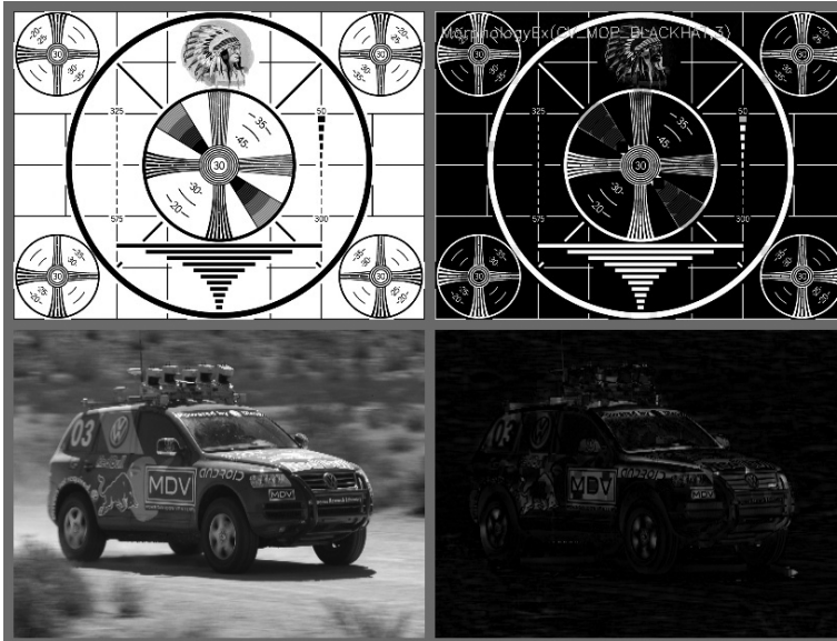
Figure 10-34. Results of morphological Black Hat operation: dark holes are isolated
