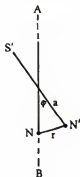
1.10 Coulomb's measurement. AB is the magnetic meridian, N the north pole of the vertical magnet, N'S' the suspended needle.
