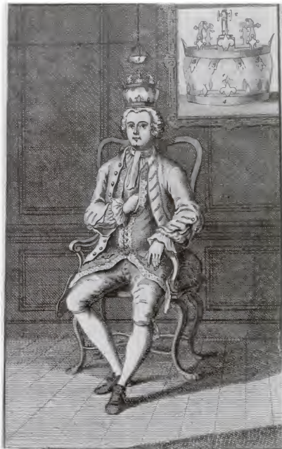
3.6 The beatification as practiced and revealed by Rackstrow, Misc. Obs. (1748). Electricity runs from a prime conductor to the plate above the crown, which is evacuated to enhance the effect.
