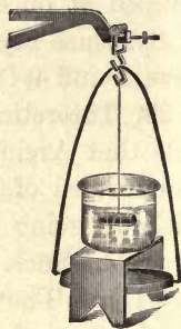
FIG. 18. Method of weighing a body under water
