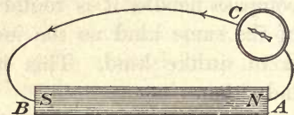
FIG. 211. A line of force set up by the magnet AB
