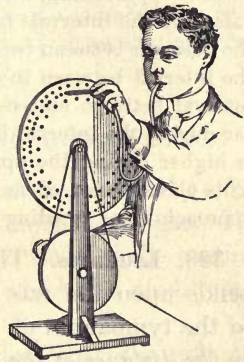
FIG. 347. Regularity of pulses the condition for a musical tone
