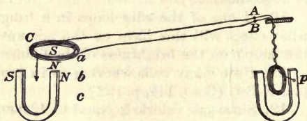
FIG. 299. Induction of electric currents by magnets
