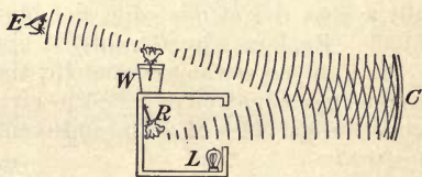
FIG. 488. Image of object at center of curvature
