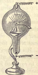
FIG. 473. Heating effect of cathode rays
