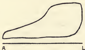
FIG. 363.—Work done during the return stroke.
