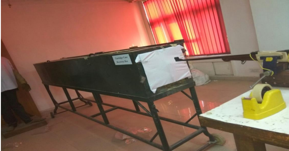
Fig. 3.6 Bullet recovery box to which the cloth sample was mounted
