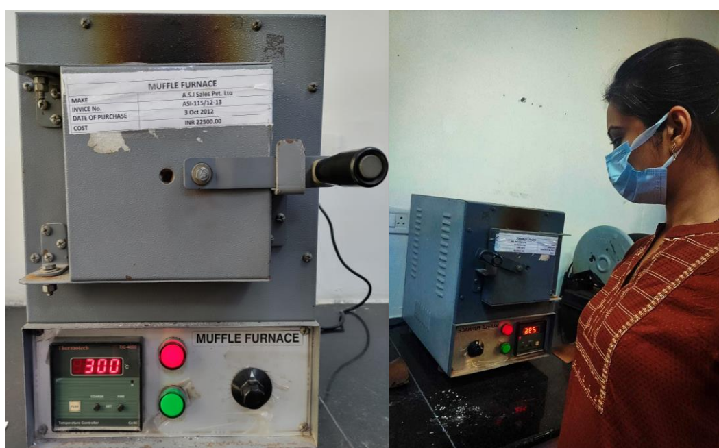
Figure 3.10: Muffle furnace used for charring the created documents under controlled temperature.
