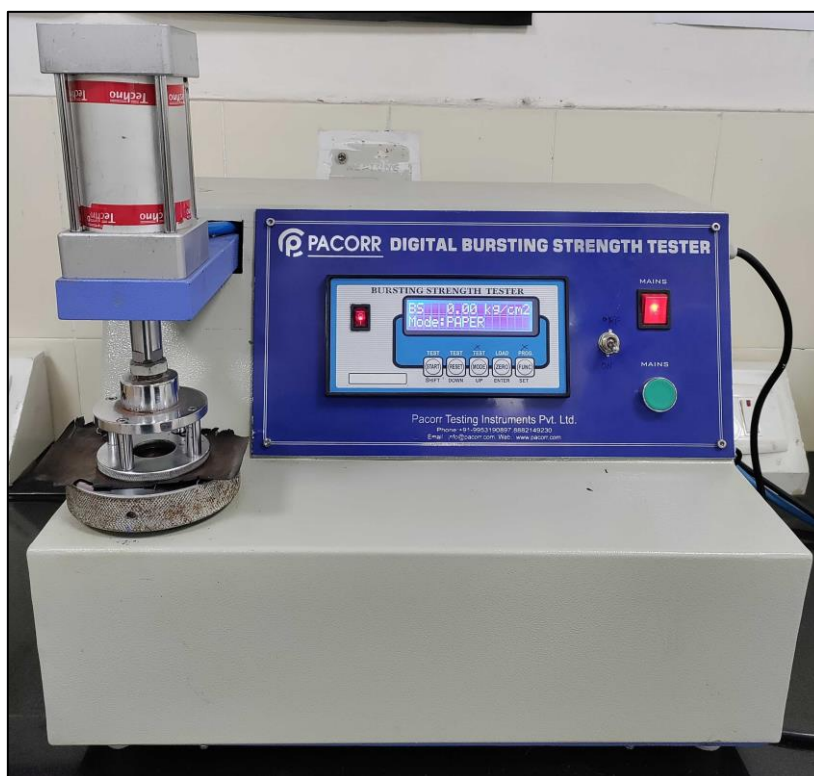
Figure 3.25: Charred Sample under analysis using Digital Bursting Strength Tester.
