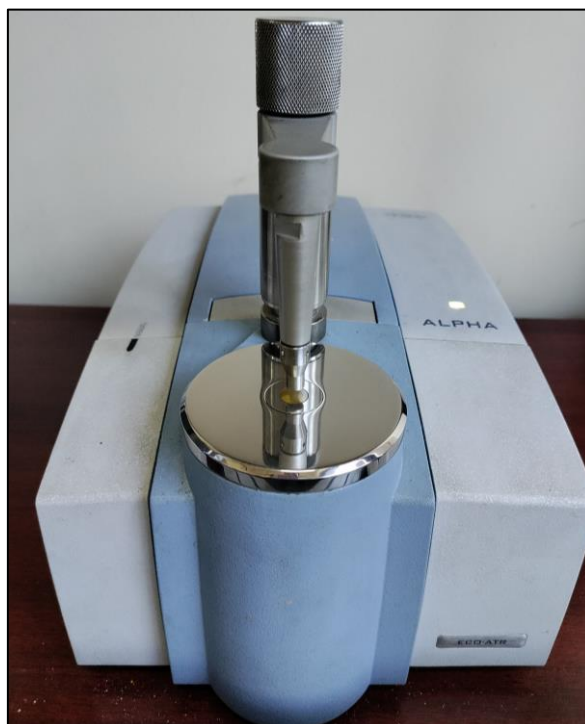
Figure 3.23: ATR-FTIR Instrument of Bruker Alpha model equipped with diamond crystal.
