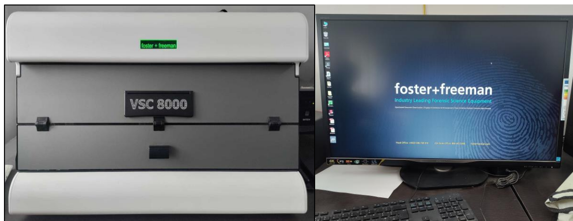
Figure 3.24: Video Spectral Comparator (VSC- 8000) with connected LCD Display Screen.
