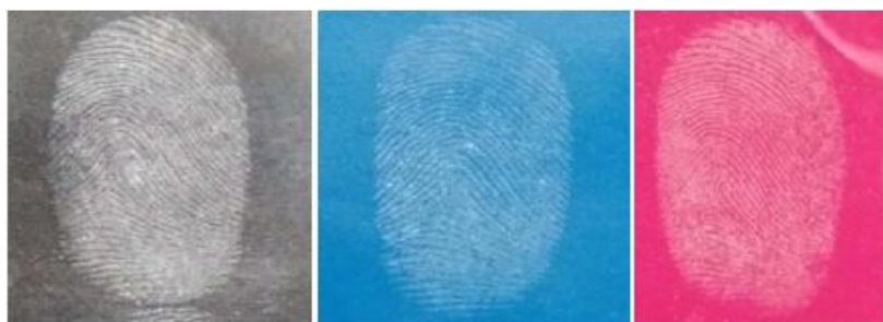
Figure 2.2: Fingerprint developed on Glass, plastic and Cardboard using Zinc Oxide nanoparticles
